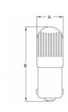
Part Number: B2A-R Serial Number: T3 1/4 MB Neon type: Indicator
